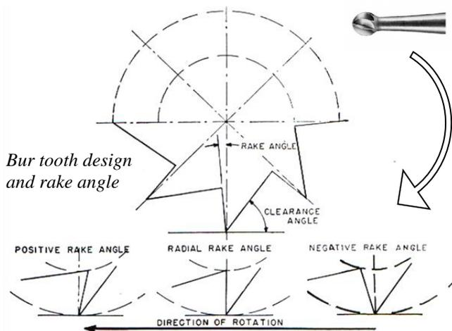
Note that in the diagram the bur is turning clockwise. The diagram shows a portion of the bur in cross-section with the teeth shown in outline. A cutting edge is shown in contact with the surface to be worked upon (the work). The side of the bur tooth which precedes is the *tooth face*: the following surface behind the cutting edge is the back, or *flank* of the tooth.
